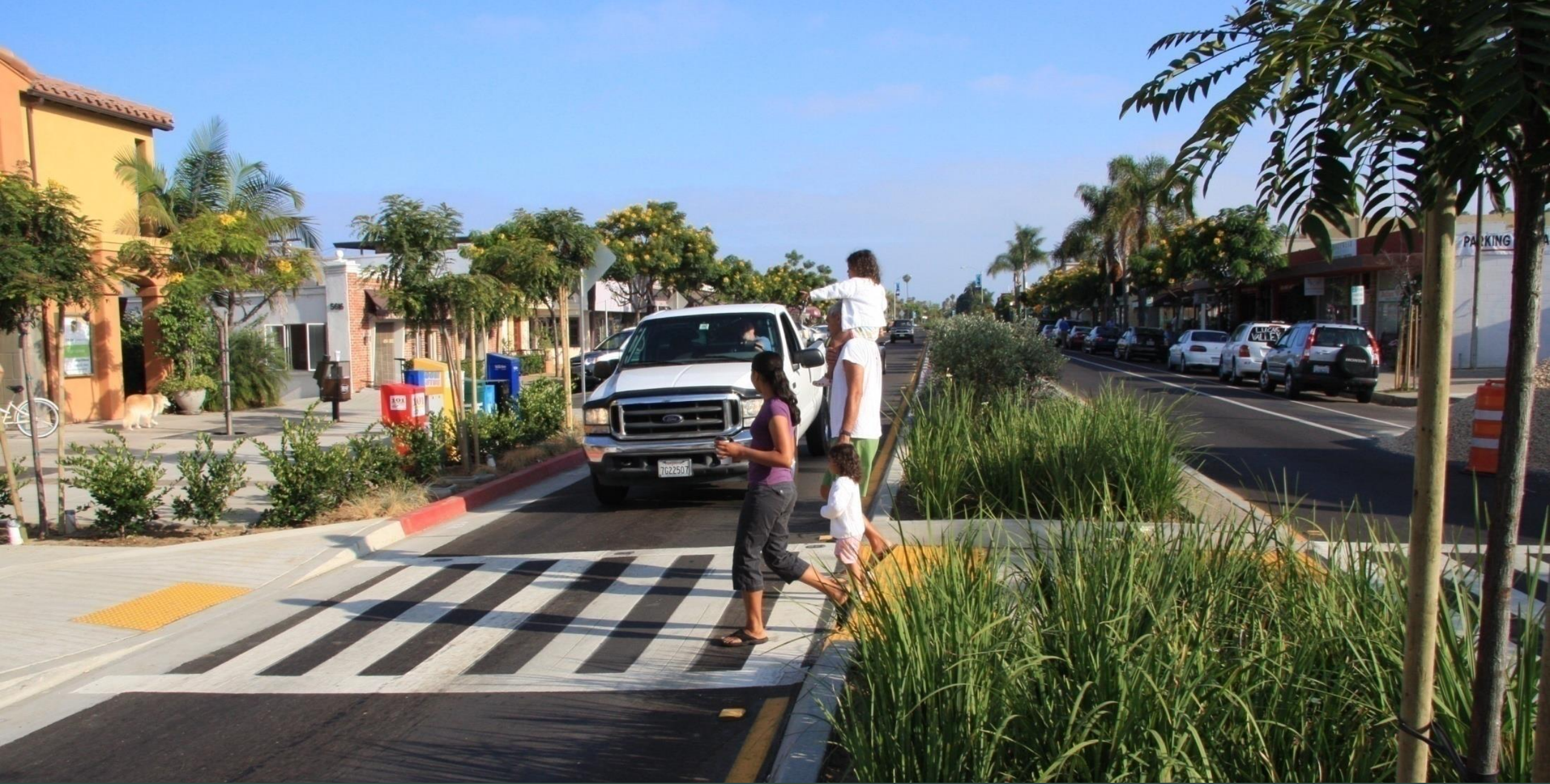
Ideally pedestrians would not need to cross more than 20 feet. With a median this becomes 14 feet.
